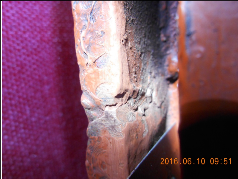
Fig. 13: NCRE Damper winding - Paint removed to investigate the area.
