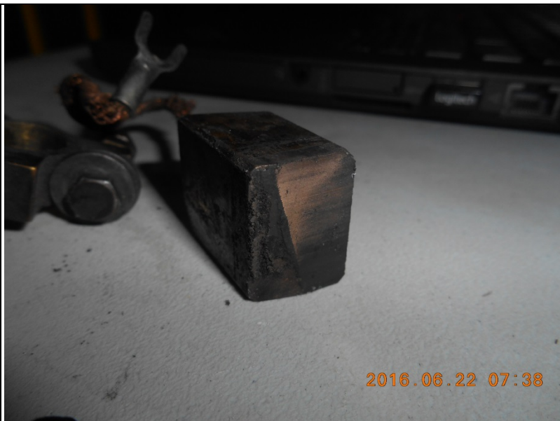
Fig. 14: Ground Brush – Requires replacement
