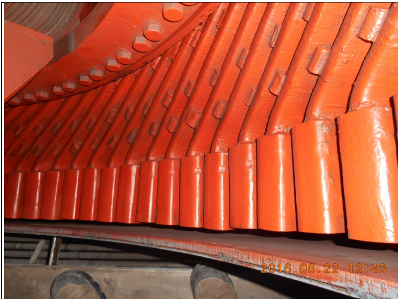
Fig. 4: Stator end turn and coil extension condition
