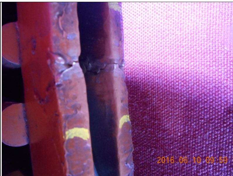
Fig. 14: NCRE Damper winding - Existing weld repair is intact
