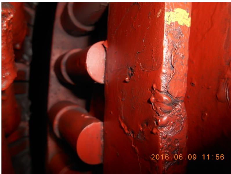
Fig. 12: NCRE Damper winding - Outer circumference at Pole 5
