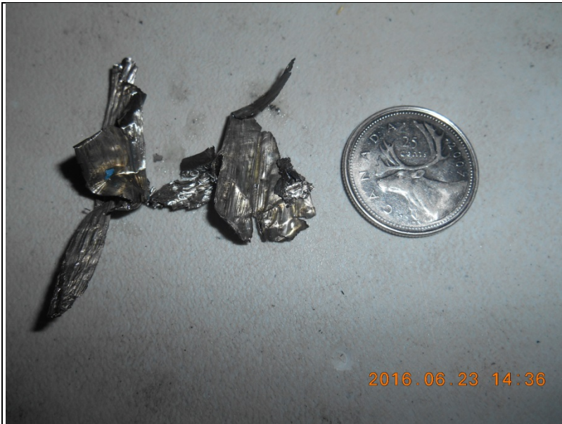
Fig. 22: Total babbitt from the bearing pedestal sump
