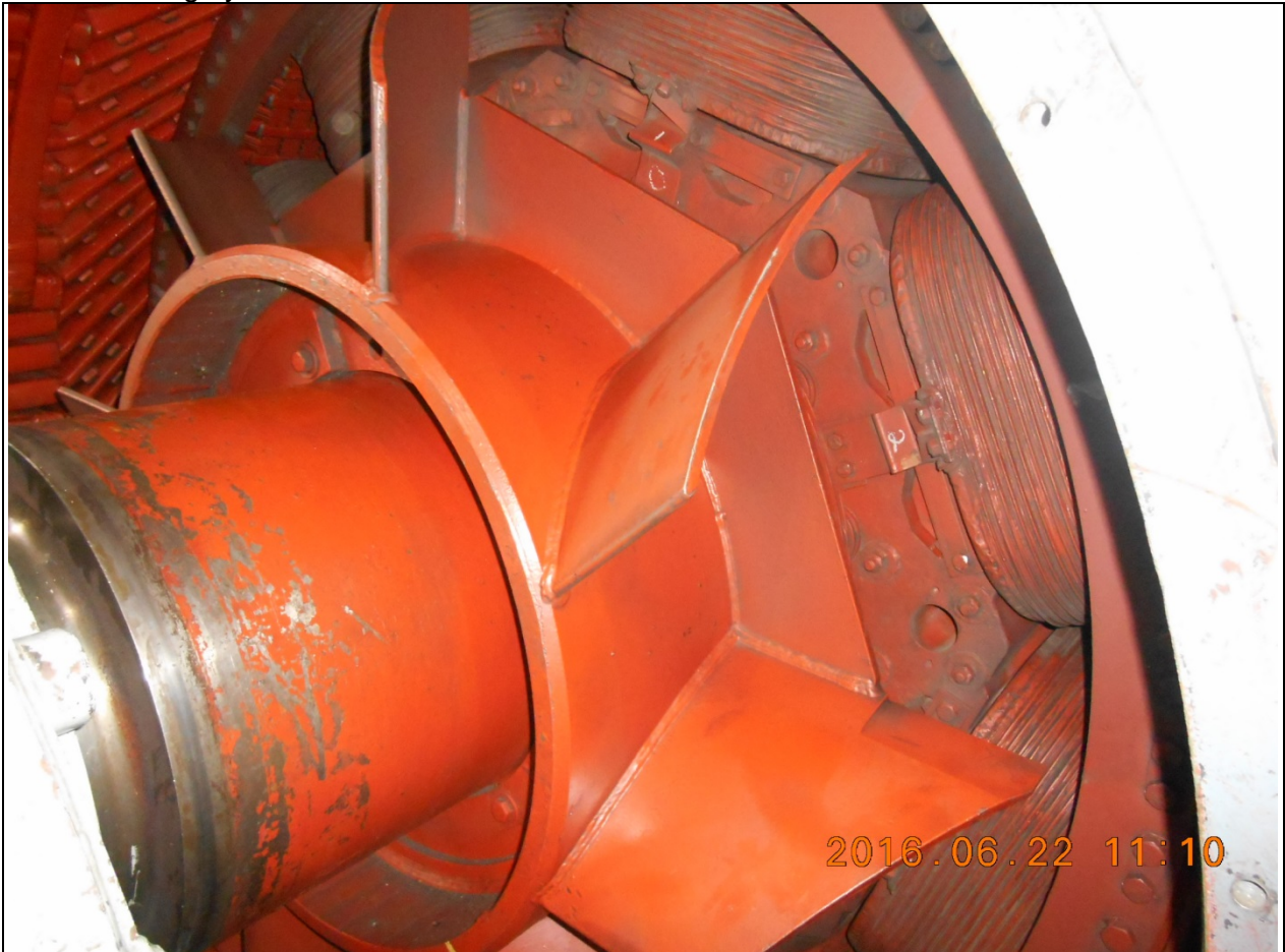
Fig. 2: Overview of Collector End - Light Dirt on Stator Winding End Turns and Rotor Poles
