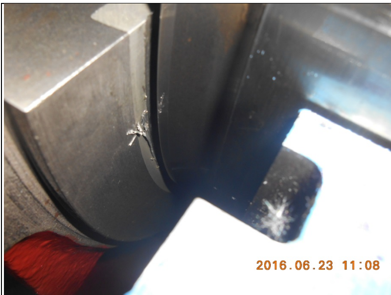
Fig. 23: Bearing damage found on outboard side
