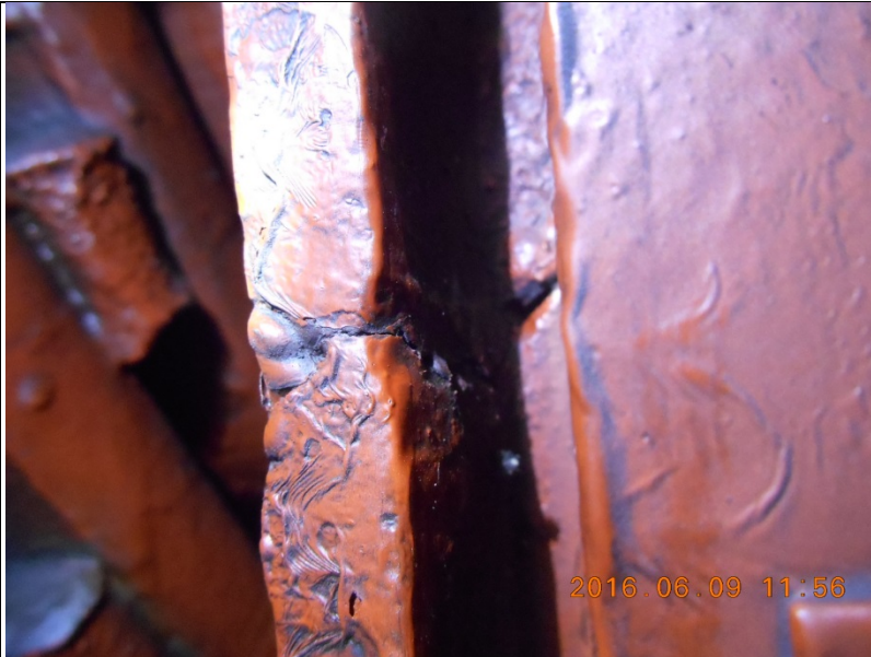
Fig. 11: NCRE Damper winding - Visual indication at Pole 5
