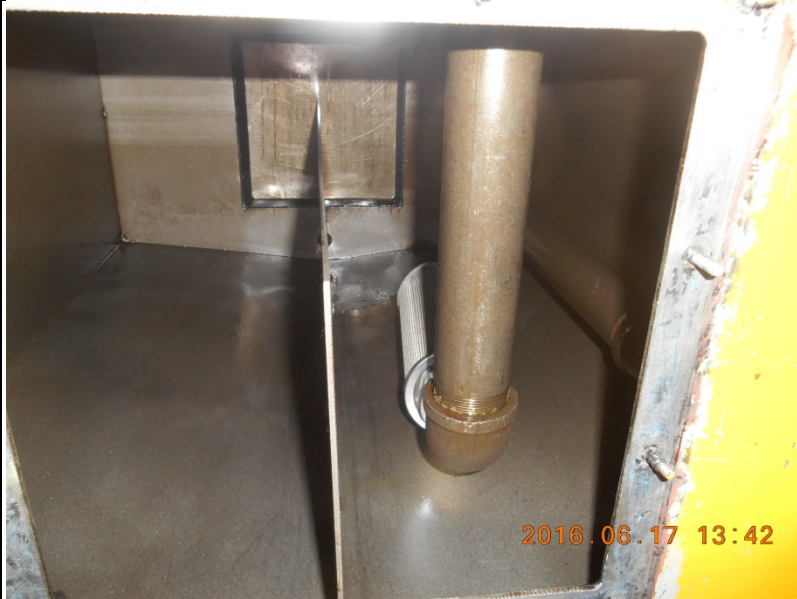
Fig. 24: Oil Reservoir cleanliness
